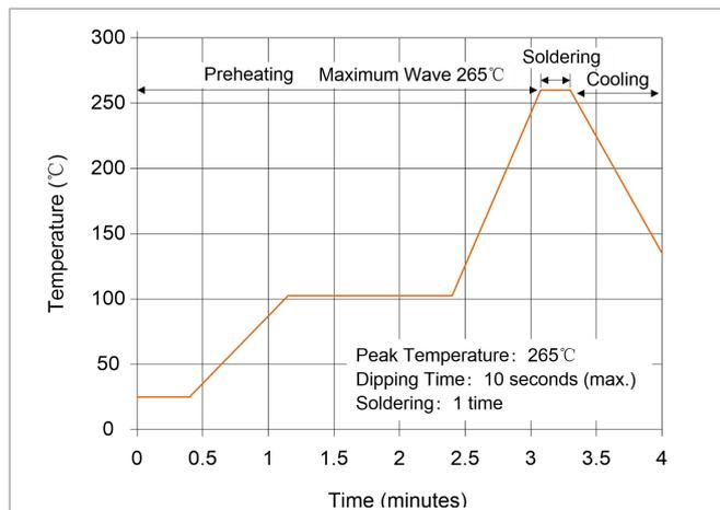
**Flow/Wave Soldering (Solder Dipping)**
